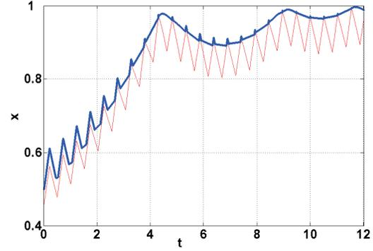
Fig. 2. Results of numerical calculations of the motion of the center of mass in a 1D horizontal system of 10 inelastic particles. Low-contrast solid line corresponds to the motion of the center of mass of the system as a whole; contrast solid line describes the motion of the center of mass of  $N-1$  inelastic particles (except the motion of the first particle nearest to the “hot” boundary of the system);  $\varepsilon = 0.95$ ,  $v_0 = 5$ ,  $dt = 10^{-5}$
