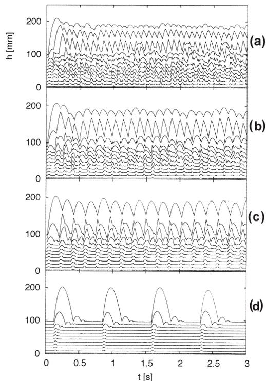
Fig. 3. Results of experimental measurements of trajectories in the vertical system consisting of 12 metallic balls obtained with the help of a high-speed digital camera. The excitation frequencies amount to: a – 13.8 Hz; b – 8.93 Hz; c – 5.61 Hz; d – 1.37 Hz
