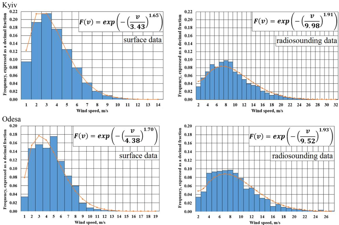
Fig. 6. Wind speed frequency with fitted Weibull distribution near the surface and at height of 1000 m at two airports of Kyiv and Odesa.
