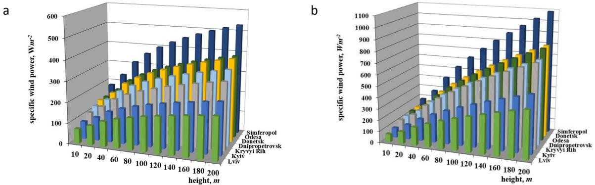
Fig. 5. Change of specific wind power in height according to a logarithmic law approximation (figure, a) and a power law approximation (figure, b) at seven airport of the Ukraine for the period of 2001 to 2008.
