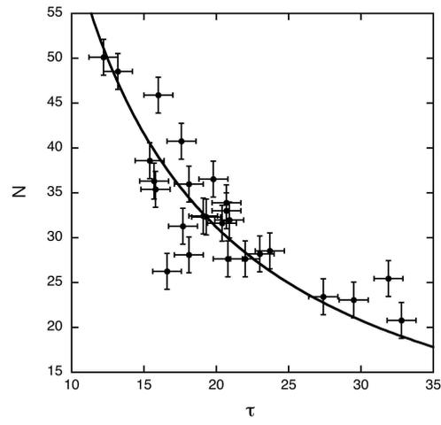
FIG. 4: The number  $N$  of avalanches in a rotating drum as a function of  $\tau$  for various powders. Error bars on measurements are indicated. The curve is a fit using Eq.(4).
