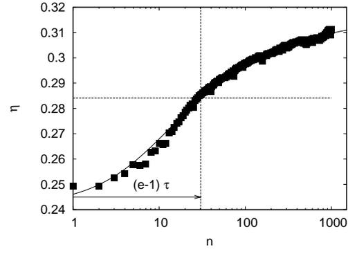
FIG. 2: Typical compaction curve of a powder in a semi-log plot. The continuous curve is a fit using Eq.(1). The relaxation parameter  $\tau$  multiplied by  $e - 1$  is shown on the plot and represents the number of taps to reach the packing fraction  $\eta = (\eta_0 + \eta_\infty)/2$ .
