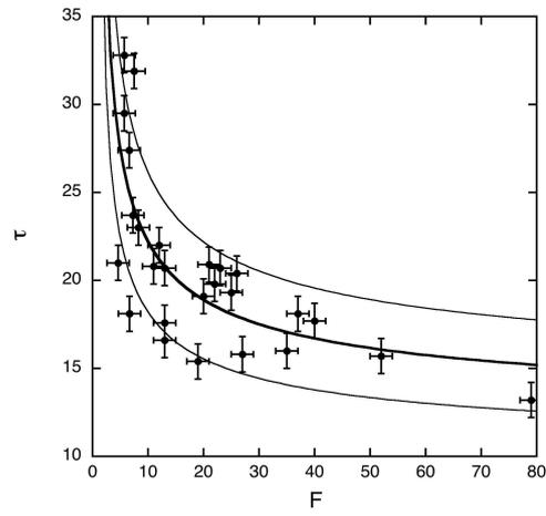
FIG. 3: The relaxation parameter  $\tau$  as a function of the flowability index  $F$  for various powders. Error bars on measurements are indicated. The thick curve is a fit using Eq.(3). Both thin curves represent the limits of the interval of confidence of Eq.(3).
