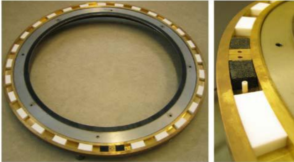
Fig. 4.1. Experimental set-up. Left: overview of the waveguide. Right: enlargement of the part close to the electric dipole antenna and the two carbon absorbers. The top brass plate covering the waveguide is not shown. The waveguide has a total diameter of 78 cm, a depth A = 1 cm and a width B = 2 cm. The frequency range of the first propagating mode is from 7.5 to 15 GHz. The length of the Teflon pieces shown is d_0 = 4 cm and their index of refraction is n = 2.08 . In this picture, the spacing between all Teflon pieces is d = 4 cm.
