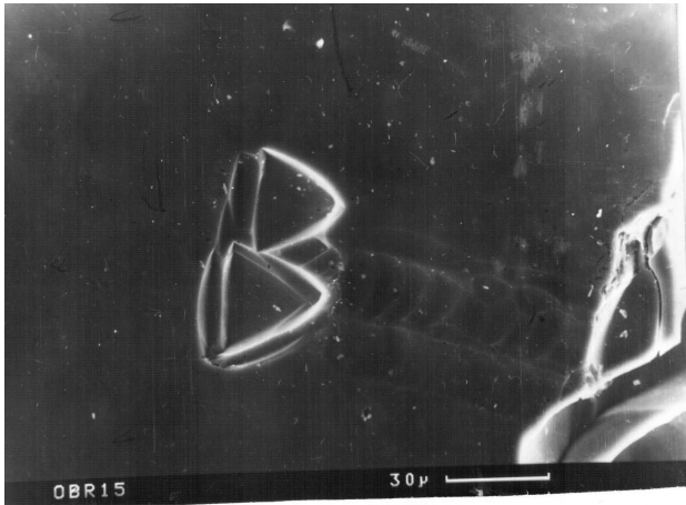
Fig.2. The SEM image of dislocation multiplication.
