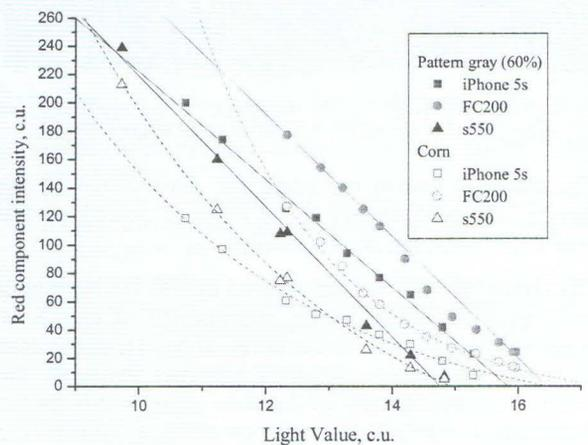
Fig. 2. Dependence of the intensity of the red color component on the value of LightValue for various models of digital cameras.
