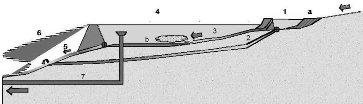
**Fig. 17.1** Conceptual dam and reservoir, designed for sustainable sediment management. (1) sediment trap, (a) delta deposit; (2) Residual water and sediment evacuation conduit; (3) Water supply to the main reservoir; (4) Main reservoir, (b) reservoir sediments; (5) Bottom outlet of the dam; (6) Fish ladder; (7) Main conduit for hydroelectric or other
