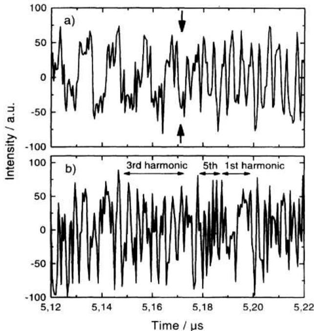
**Fig.5. Time series of intensity in GaAs / GaAlAs Hitachi HLP1400 laser (experimental data by Fischer et al (Marburg, Germany, 1994)/**
