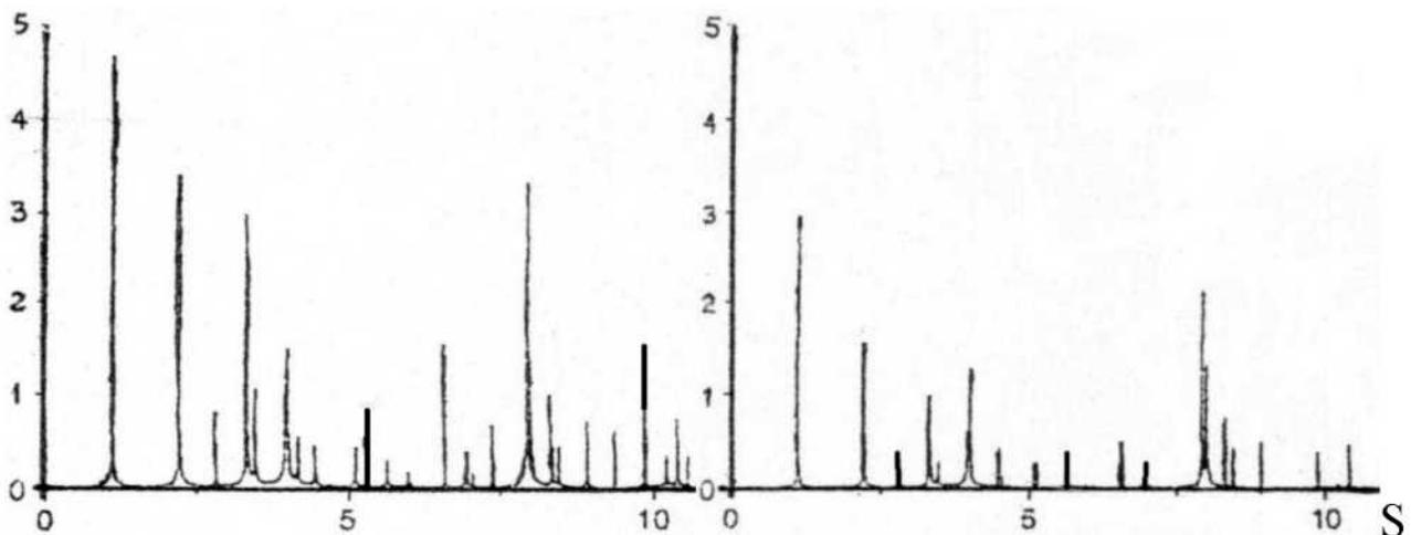
Fig.2. The power spectrum of Rb: : a- in a magnetic field (f = 0, the electric field is absent); (b) in a static magnetic field and oscillating electric field f = 0.0035 (our data).
