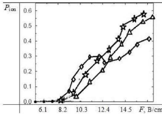
**Fig.3. Our data on the dependence of ionization probability for atoms Li in the initially prepared states with  $l_0=0, m_0=0, n=63,67,69$  on the field strength  $F$ :  $n=63$  ( $\diamond$ ),  $n=67$  ( $\triangle$ ),  $n=69$  ( $\star$ ).**
